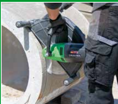
precise cutting depth adjustment (accessory)
